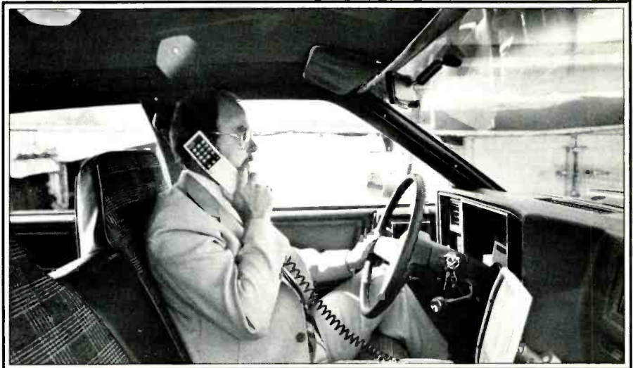
The latest mobile phones have touch-tone calling and also automatic ringing. Each unit can operate on several different channels.
